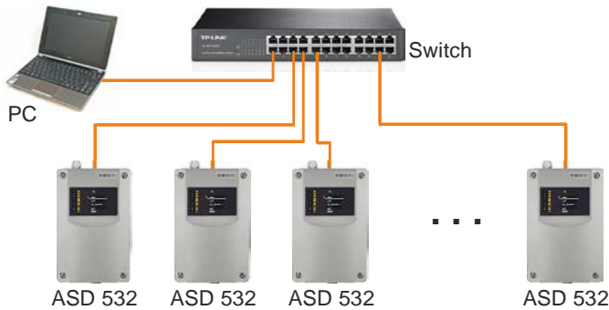
Fig. 53 Design of an Ethernet ASD network
